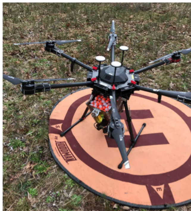
DJI Matrice 600 Pro drone with attached hopper filled with dragon eggs.
